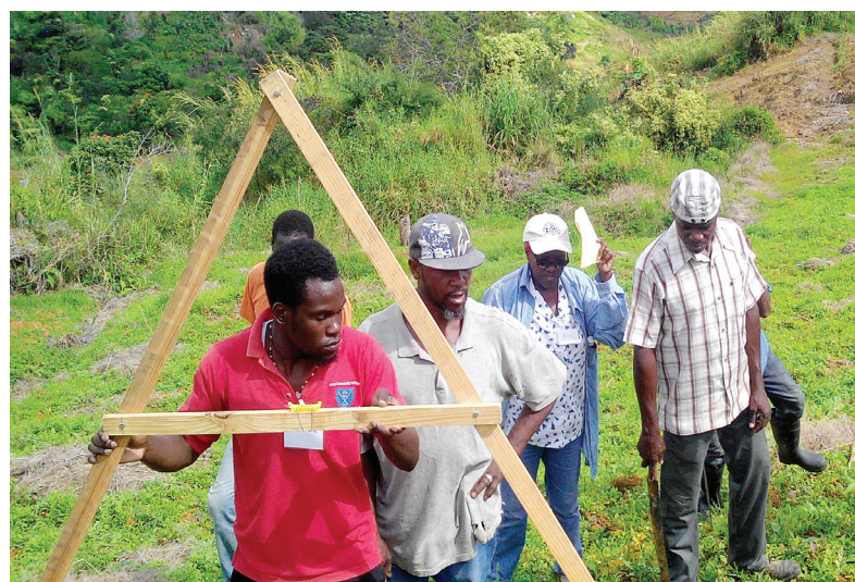
Demonstration of proper Land Management Practices using an A- Frame.
