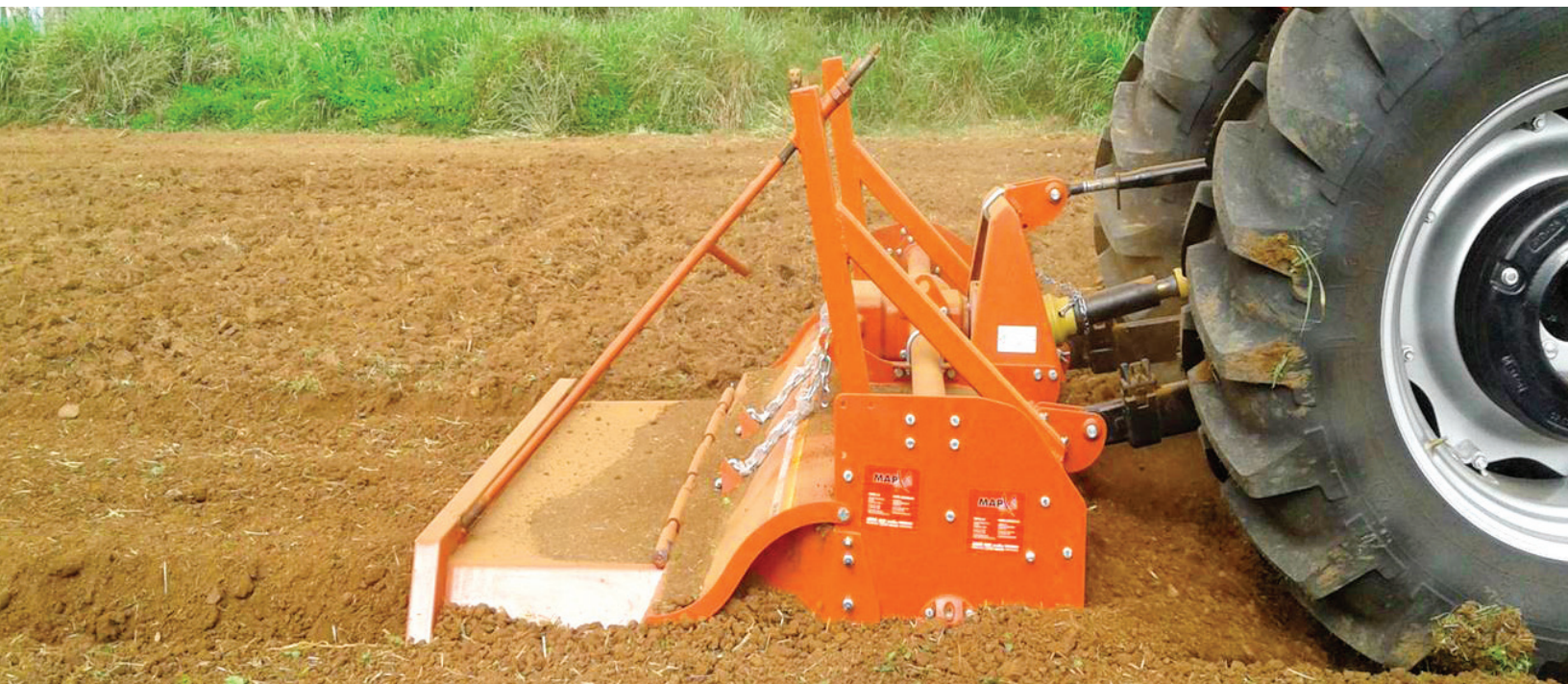
Land preparation conducted using Rotobedder Implement.
